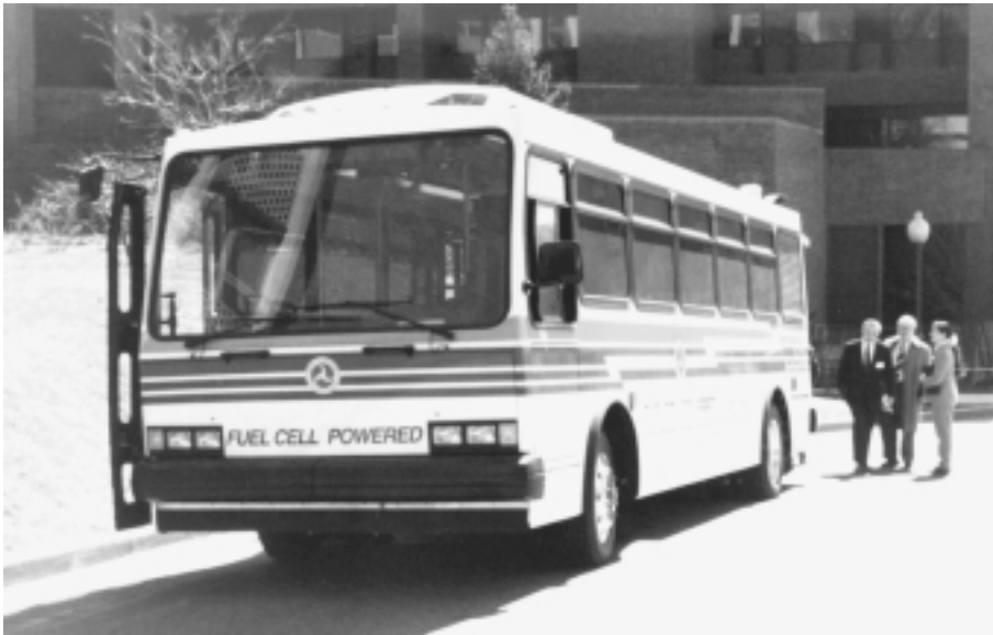
Non-polluting fuel-cell bus (developed at Georgetown University) is one application of NEICES technology which could be commercialized at the New Birth facility.
